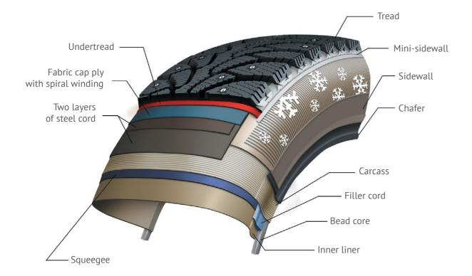
The tread is a wear part of the tyre that comes into contact with the road. It is made of wear resistant rubber showing excellen grip characteristics on any road surfaces.
